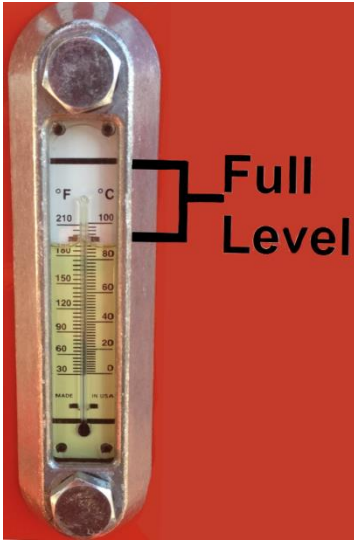
Fig. 5-1 Hydraulic Fluid Level and Temp. Gauge
